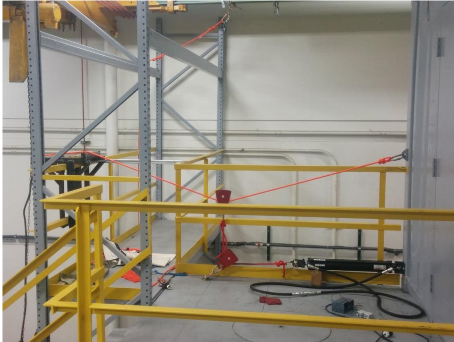
Figure 2: The test set up utilizing a vector pull to produce travel in the sample
